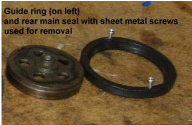
Guide ring (on left) and rear main seal with sheet metal screws used for removal
