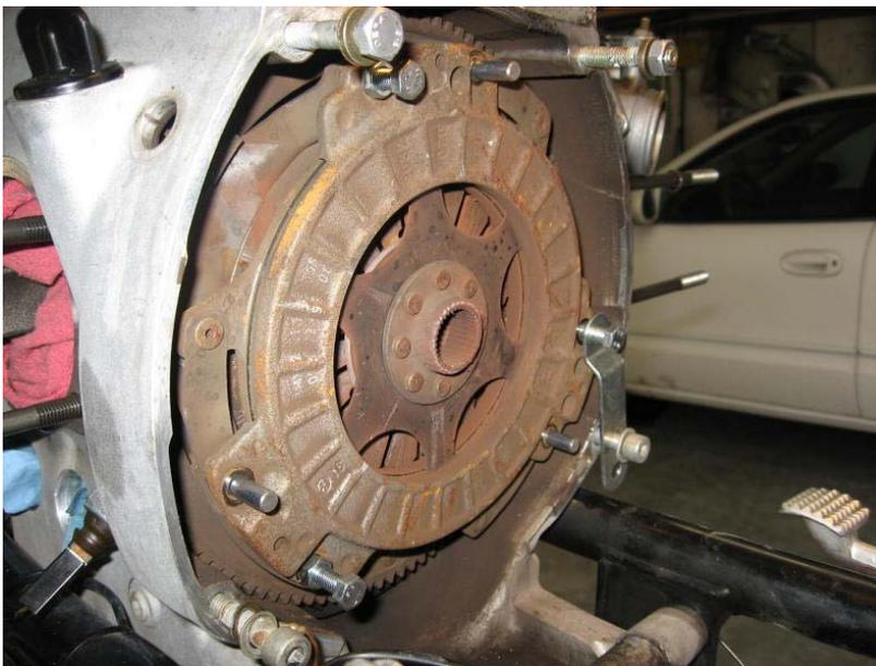
This shows two of the three clutch spring compression bolts and nuts (12 o'clock & 7 o'clock, my home-made flywheel brake (3 o'clock) and my three home-made clutch removal/mounting studs (the smooth ones at 1, 4 and 8 o'clock). The flywheel brake bolt is finger tight and will be removed to install the third compression bolt and nut.
