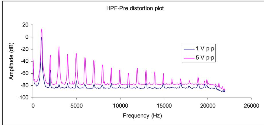
At 1 V p-p, The second harmonic is at  $\approx -55$  dB, and the third harmonic at  $\approx -78$  dB. The rest of the harmonics are consistent with the distortion floor of my measurement system. Pure second harmonic distortion at -55 dB corresponds to a THD of 0.17%, which is quite respectable for a Class-A circuit. This is with an input voltage of 1 V p-p.
