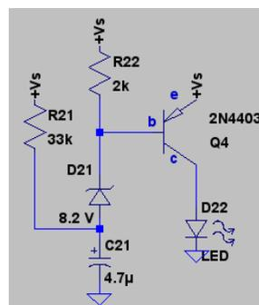
There's enough variation in Zener diodes that some of them are unsuitable. I have a test jig with a 1k resistor in series with the Zener, and measure the forward voltage of each diode. With the 1N5237B diodes, most come in around 7.8 V in my test, and I throw away the ones that are much higher than that. This appears to result in a "flash" threshold of around 8.5 V, which seems like a decent level. Since 9-V alkaline
