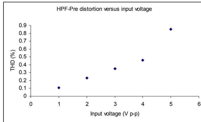
Distortion rises with increasing amplitude. But unlike an op amp circuit, the dynamic range is not a hard upper limit. You can push beyond this range, at least on the transient at the front end of a plucked note, with minimal audible effect. I expect this circuit to be quite forgiving.
