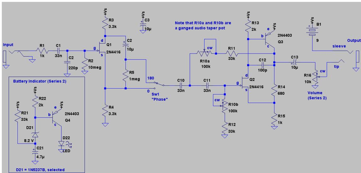
Q1 is a classic JFET phase inverter circuit. Since negligible current flows through the gate of Q1, equal currents flow through R3 and R4. The signals at the source and drain of Q1 must be of equal amplitude but opposite phase. A SPDT switch selects one of these signals – it is the phase switch. C2 and R5 hold the DC offset of these signals equal, so there is minimal "pop" when you flip the switch.
